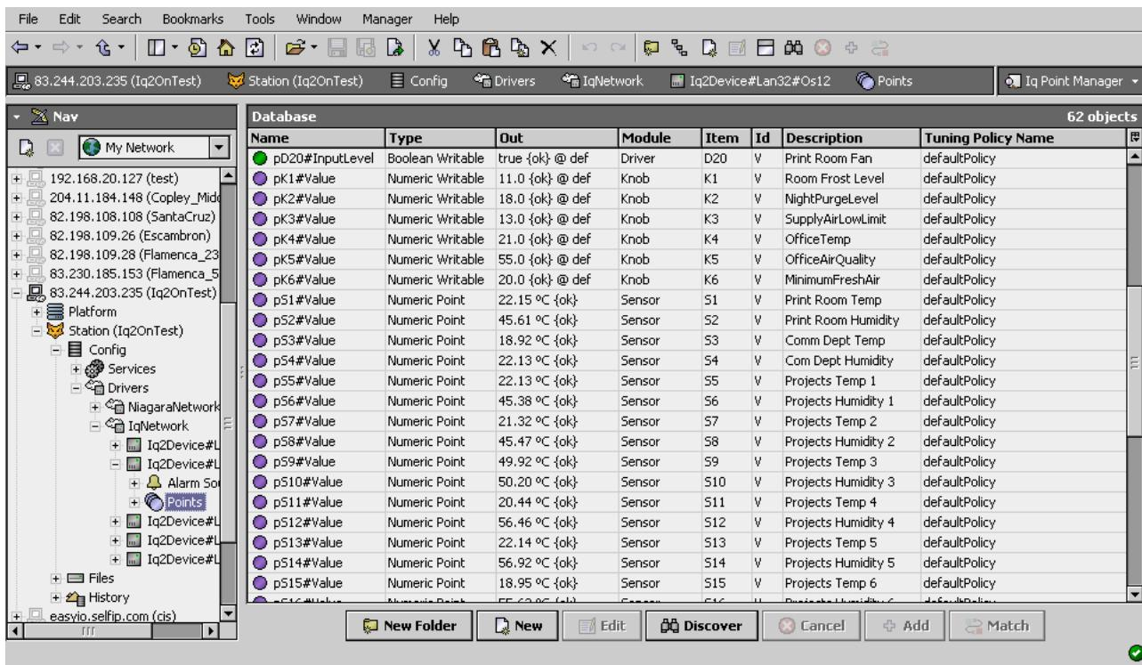
The “New Folder”, “New”, and “Edit” buttons are not unique to the Iq Device Manager, and are explained in the “Niagara AX User’s Guide” in the “Driver Architecture” section. The “Match” button is not used for the Trend IQ driver.
