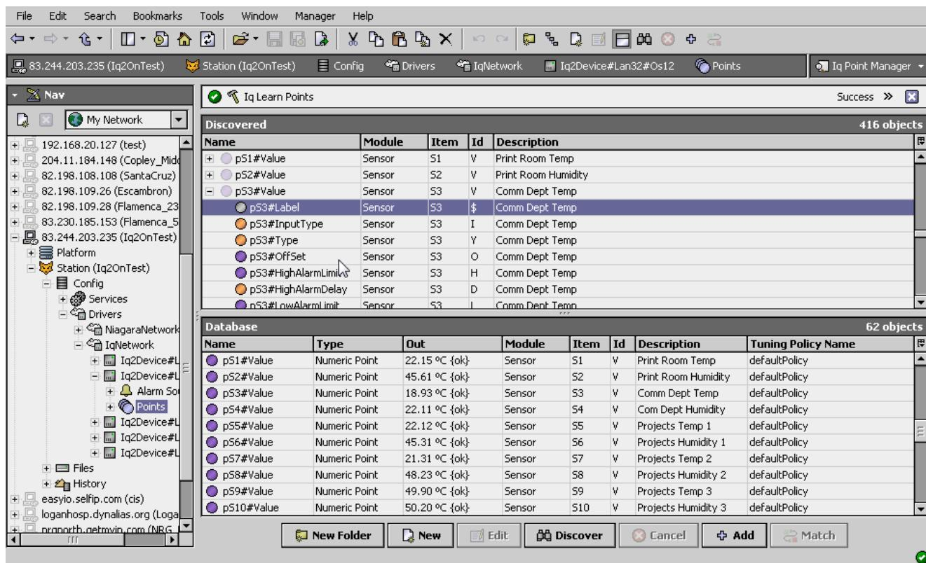
Single or multiple points can be added as control points with IqProxyExt extensions by selecting the discovered row(s) in the top pane, and clicking add. Doing so will cause the “Add” dialog box to appear. Once the point(s) are satisfactorily edited, click “OK” to create the proxy points corresponding to the point property.
